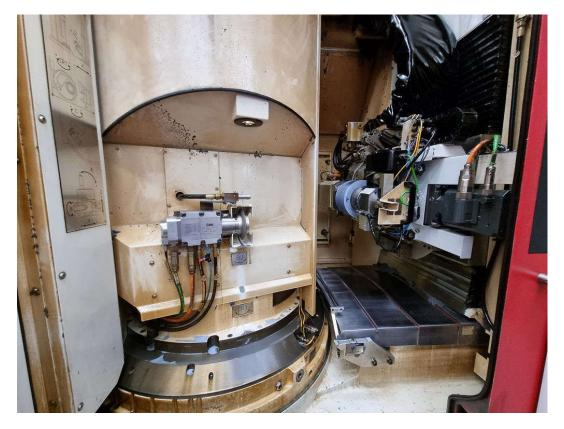
The KX 500 FLEX gear grinding center is suitable for both generating and profile grinding of gears and pinions. Workpieces up to a diameter of Ø 500mm and a length of max. 1,000mm can be machined on the machine.
